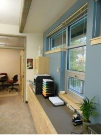
When providing natural daylight to spaces, the project must consider glare, energy efficiency, and heat gain. All factors can be affected by adding window area. Although windows were added on the south and west elevations where heat gain can be a particular concern, the existing building form provides protection. Covers over the exterior walkway block the high summer sun and shade window surfaces when heat gain could be a serious problem.
