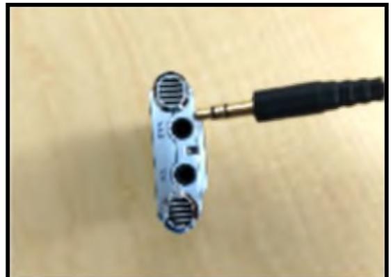
2. Put the other end of the audio cord into the audio in (microphone) jack of your computer.
